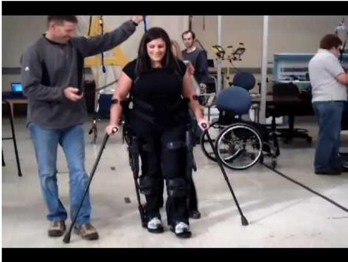
Alyson Roth wears the device developed by Ekso Bionics, which is a battery-powered, robotic exoskeleton, designed to aid wheelchair users and those who have suffered from spinal chord injuries to stand and walk. (californiaandme on Youtube)
